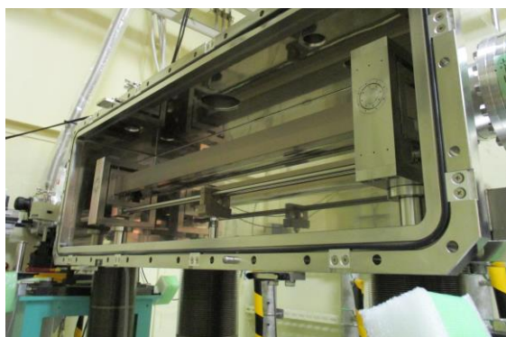
Fig. 4. Ir-coated cylinder mirror of BL40B2 experimental hutch.
