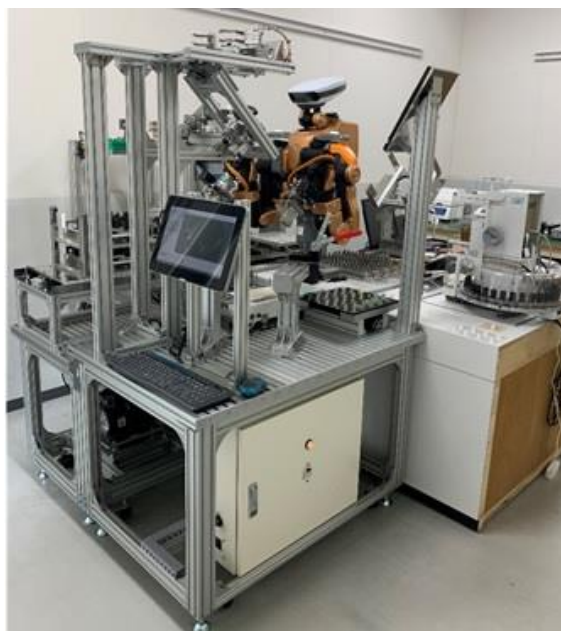
Fig. 1. Photograph of the automatic pellet sample preparation system for XAFS measurement.
