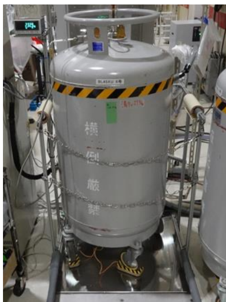
Fig. 2. Self-pressurized tank installed on a load cell.
