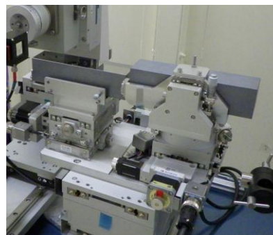
Fig. 4. Photograph of multilayer focusing mirrors in the K–B geometry for 100 keV X-rays.
