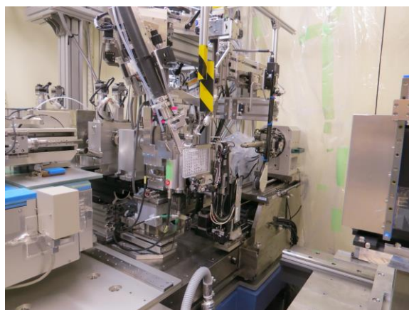
Fig. 1. Plate-scan goniometer installed on the BL26B1 diffractometer.
