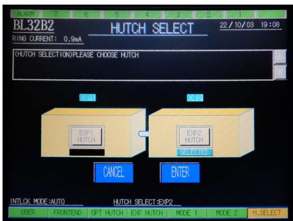
Fig. 2. Appearance of a graphic control panel for HUTCH SELECT. Users can switch the active experimental hutch without closing MBS.
