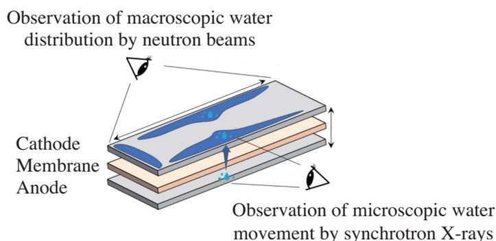
Fig. 1. Concept of multiscale water visualization inside PEFCs.
