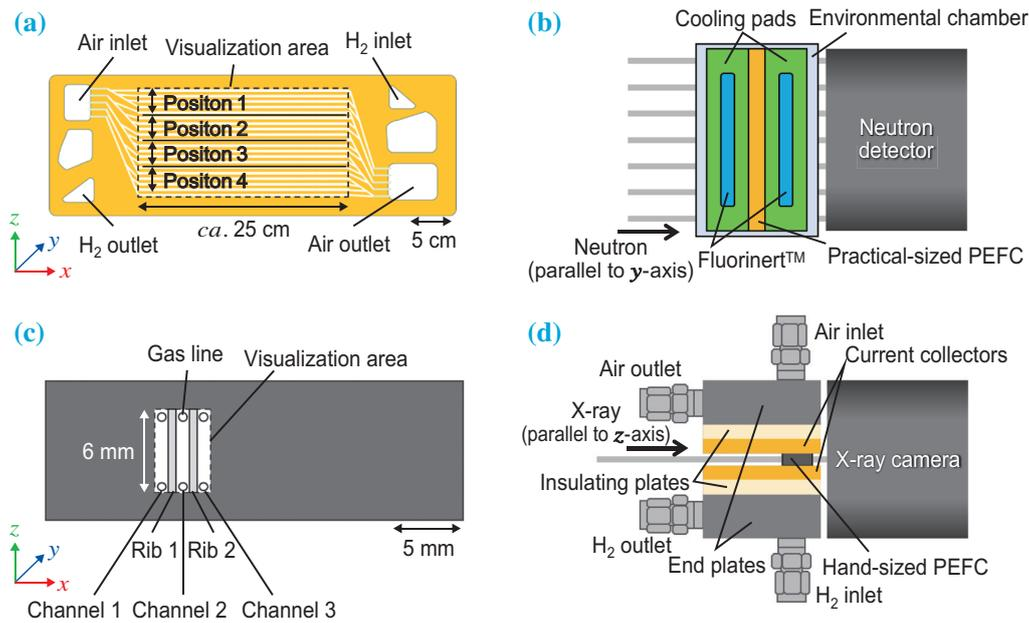
Fig. 2. Experimental setups for *operando* (a,b) neutron and (c,d) synchrotron X-ray radiography. [1]
