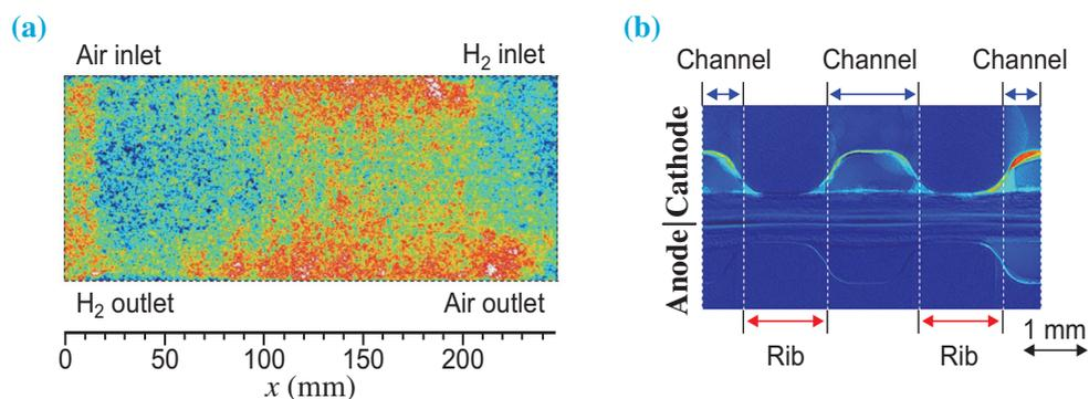
Fig. 3. Water distribution in (a) planar and (b) cross-sectional direction of PEFC. Blue and red indicate low and high water contents, respectively. [1]
